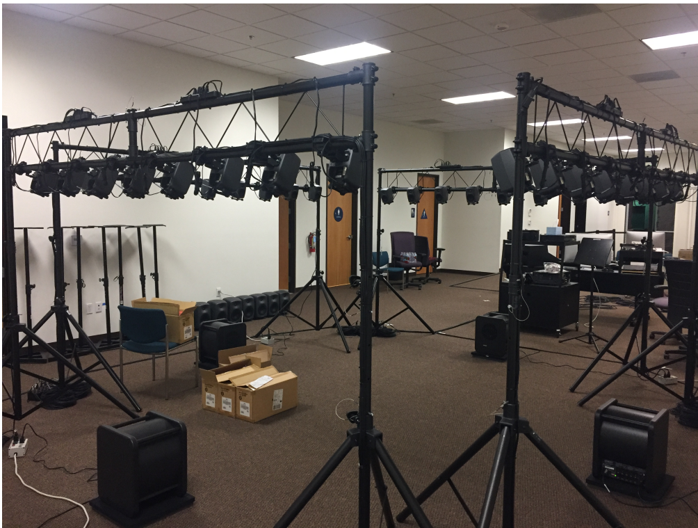
32-channel immersive sound system – back view
